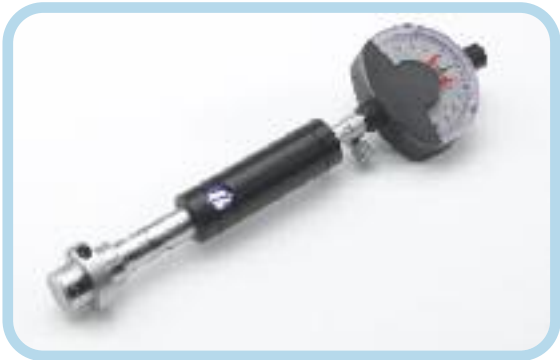
SmartPlug with depth stop
