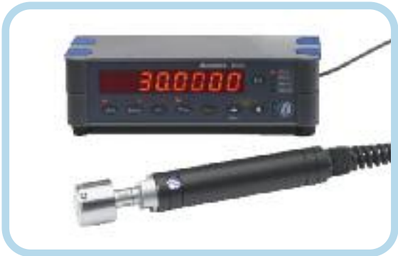
SmartPlug with transducer holder and D50S digital readout
